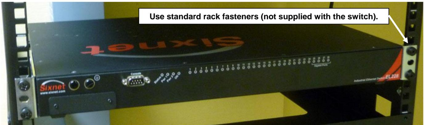
The above image shows an EL228 in reverse/rear style arrangement (ports and power in the back) Mounted in a typical 19" rack, prior to wiring.
