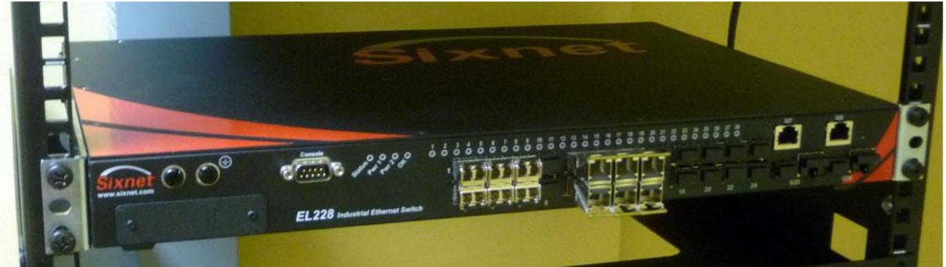
The above image shows an EL228 in front style arrangement (ports in front and power in the back) mounted in a typical 19" rack, prior to wiring.
