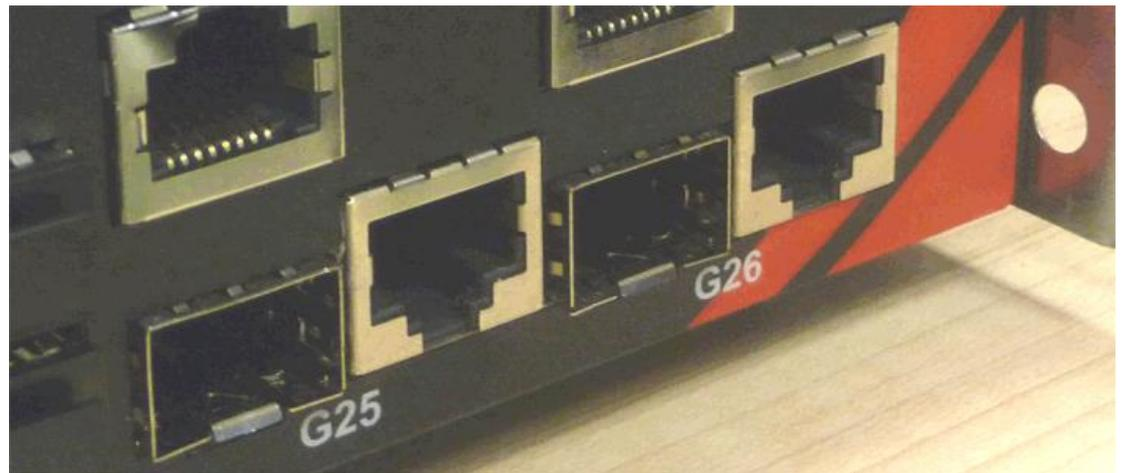
**Note:** For each of these ports (25 and 26) you can only use one of the connectors (RJ45 or SFP) at a time. If you connect to both at the same time then neither connector may work.
