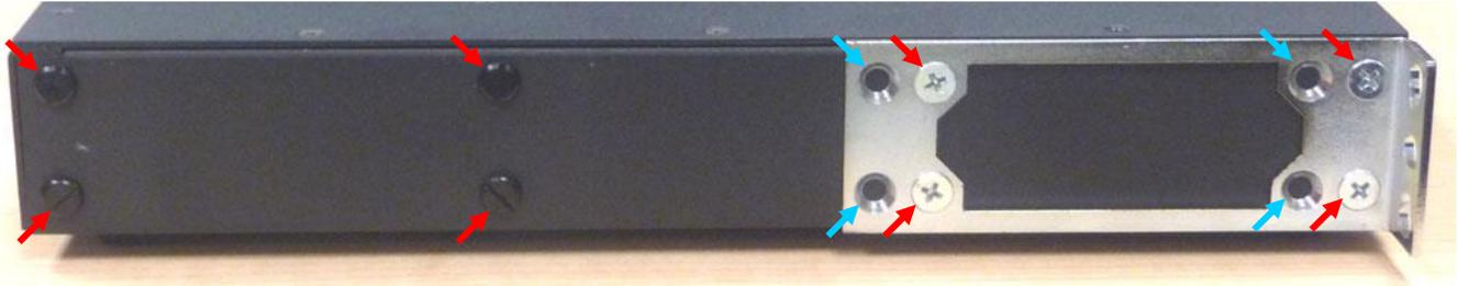
There are eight threaded inserts (see red arrows above) on each side of the switch that allow the brackets to be mounted in numerous positions for the best fit in your rack. The brackets also have extra holes (see blue arrows above) allowing them to be shifted right or left 1/2 inch. Use the supplied screws to mount the bracket in the desired position. Plastic screws are also provided to plug the unused holes. See below for possible mounting positions.
